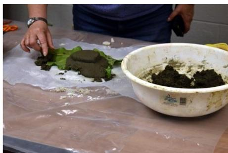
Mix two parts fine sand with one part Portland cement. Add enough water to make it the consistency of stiff cookie dough. Starting at the center and working to the edge, start adding small handfuls of the cement pressing them onto the back of the leaf. Be careful to work it into the veins of the leaves. The cement should be  $\frac{1}{2}$  to  $\frac{3}{4}$  inch thick in the center tapering to  $\frac{1}{4}$  inch at the edge. Add an extra flat area in the center to serve as a base if desired.
